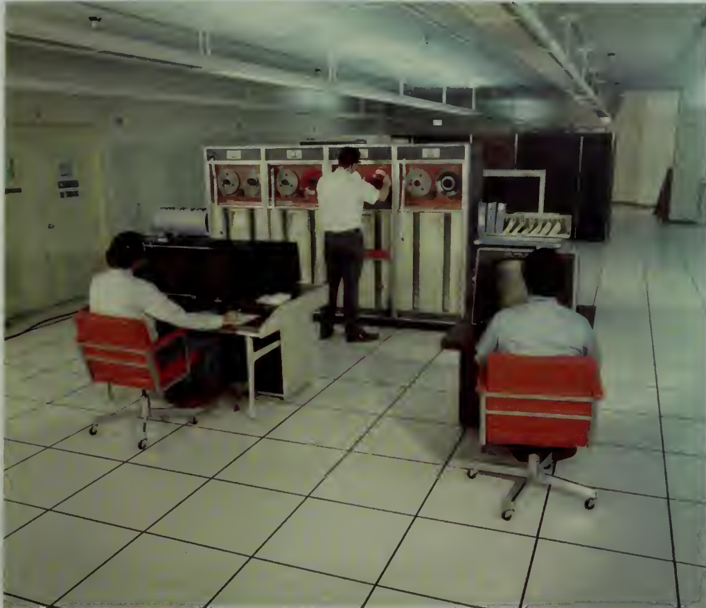
Fig. 3-2. Computer systems play vital roles in missile defense. One such system for Site Defense was this CDC-76-computer, which was operated and maintained by the control consoles in the foreground-May 1974.
